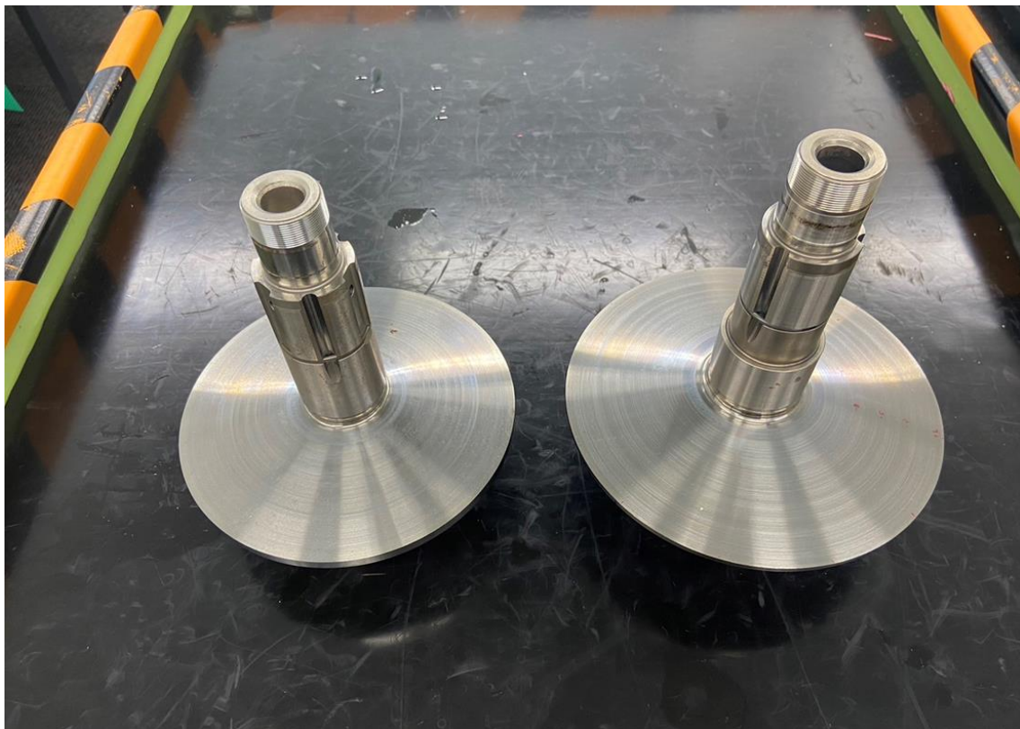
Pulley shaft that took on the challenge of making the shaft thinner (left: CVT-XS, right: CVT-X)
