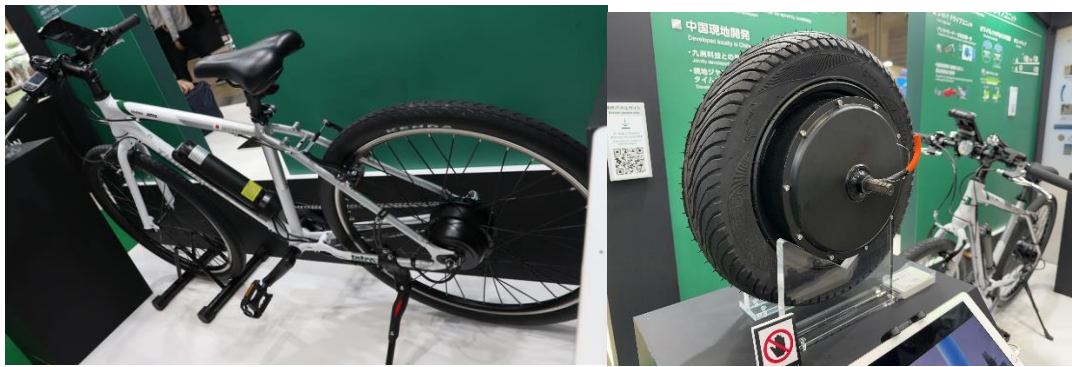
(From the left) Electrically assisted bicycle with drive unit, 2-speed automatic in-wheel motor drive unit for electric bikes
